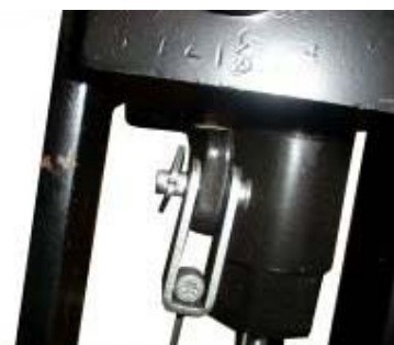
b) Secure the chain into the pump block using cotter pins and the axle.
