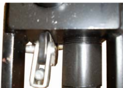
b) Secure the chain into the pump block using cotter pins and the axle.
